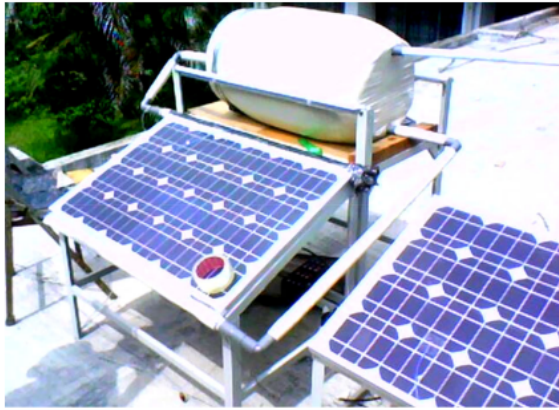
Fig. 1 Water-cooled PV panel (left) and standard PV panel (right)
