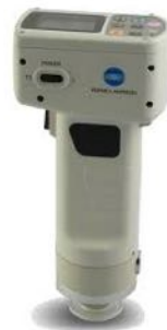
Figure 2: Chromameter CR-400 Konica Minolta to analyze degree of whiteness
