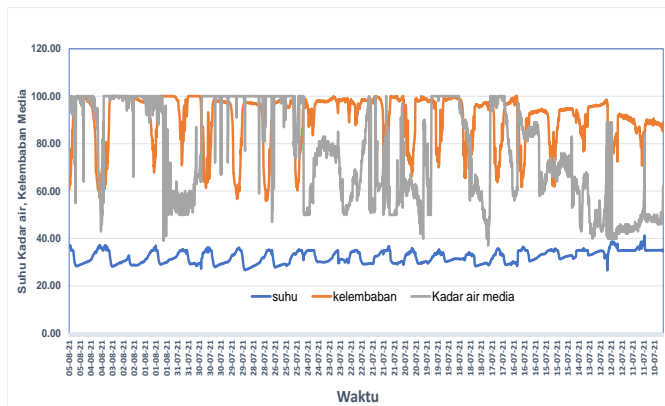
Figure 4. Condition of air temperature, RH, and moisture content inside FRP House
