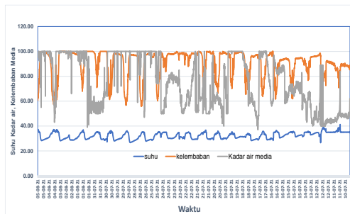
Figure 4. Fluctuation of air temperature, RH, and moisture content inside FRP House
